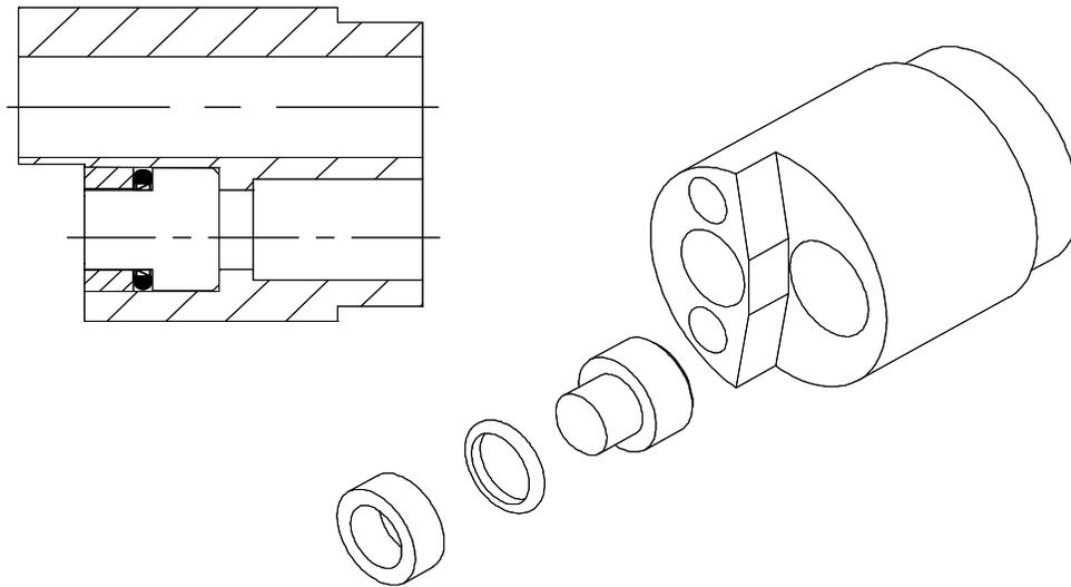
Figure 1: Cross section and exploded view of Axiom's welded metal seal assembly as used in the FPT-850 transmission probe.
