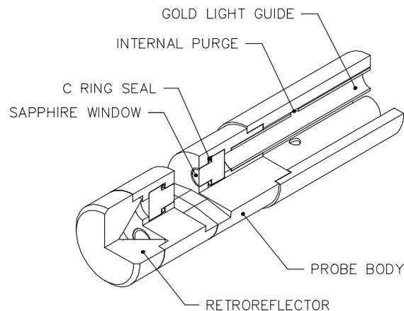
Figure 2: Breakaway view of the FPT-850 probe tip.
